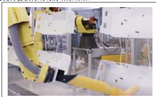
Figure 2: Gun with 45 ° angle nozzle for axial connection to the robot arm
