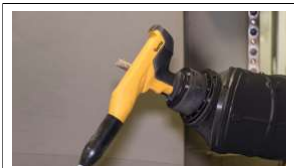
Figure 1: Gun with angular displacement for connection to the robot arm
